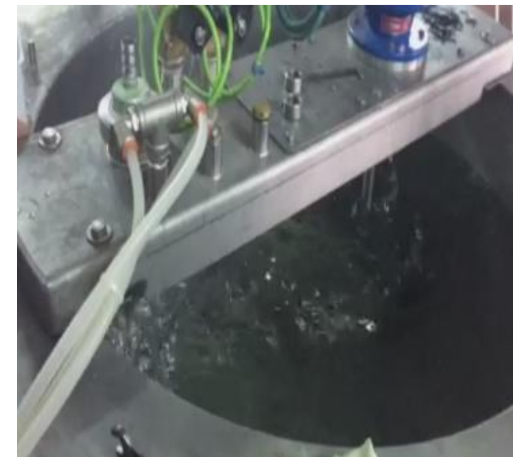
Hydrolysis in a pH-stat reactor (300 L)
