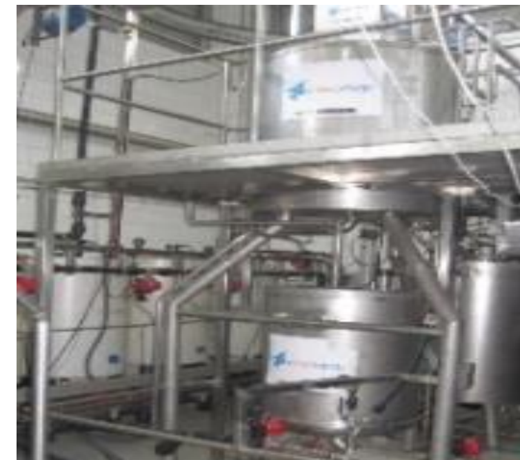
Hydrolysis in a pH-stat reactor (300 L)
