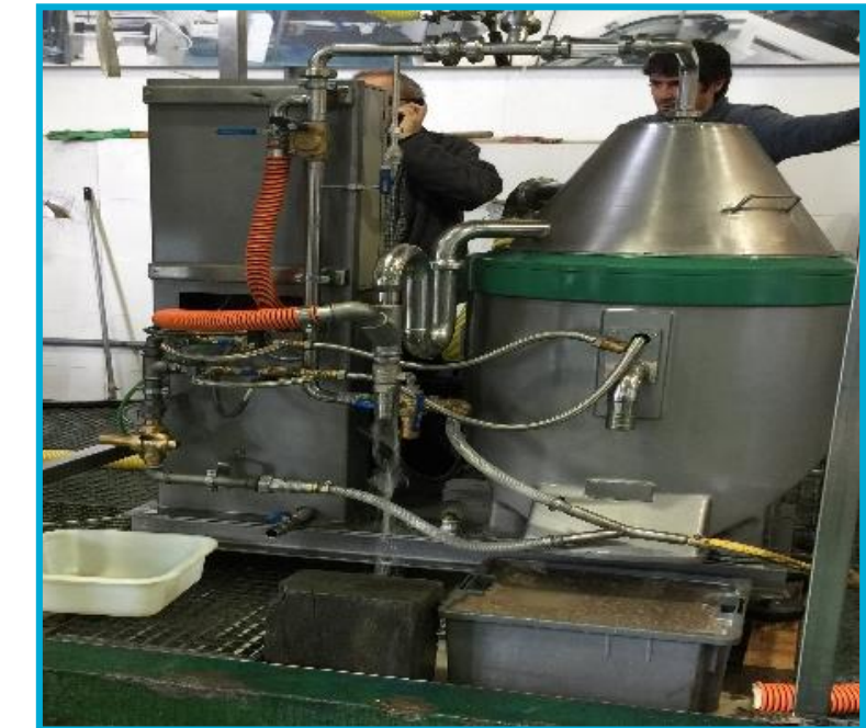
Separation of aqueous FPH and fish oil by centrifugation in a tricanter
