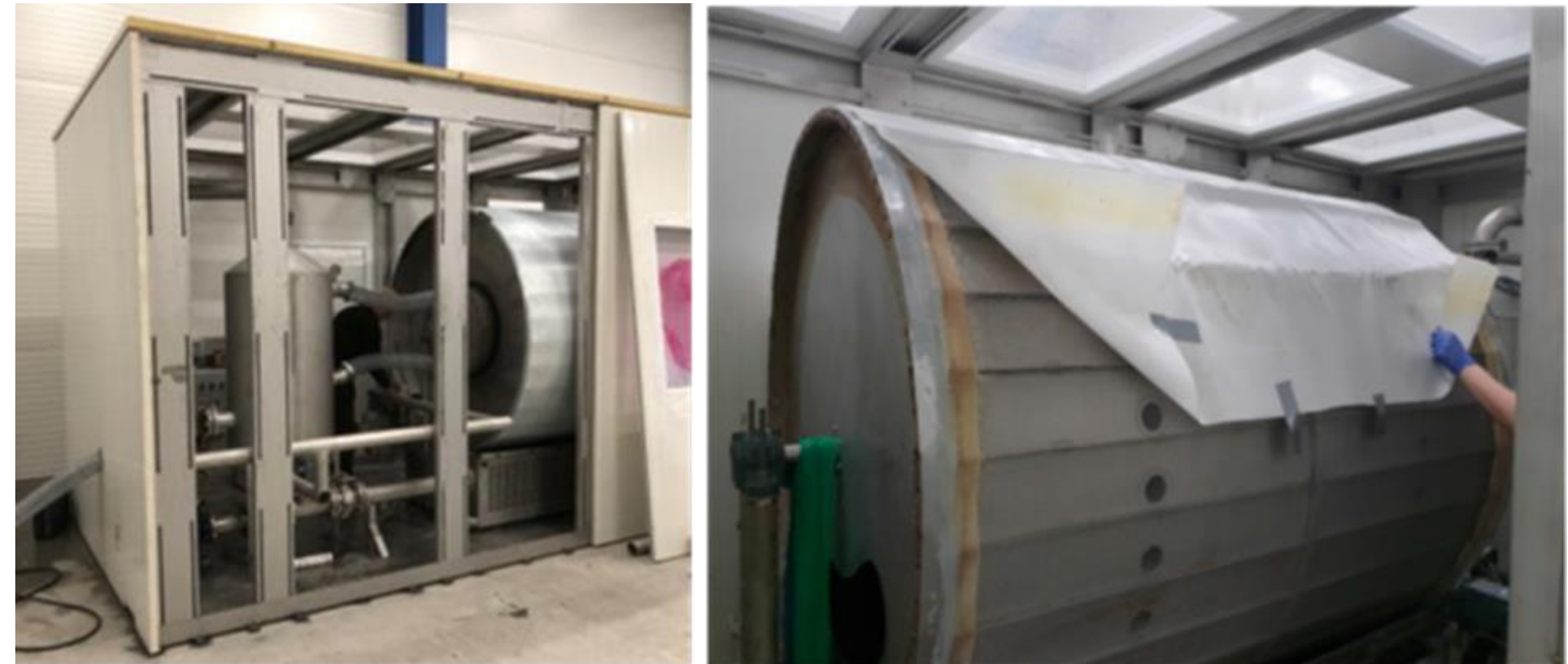
S3 filterdryer demonstration unit as produced by Salten Havbrukspark/LS Optics AB. Right frame show the details of the filter during change of filter cloth.
